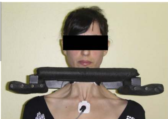
Fig. 2. EMG during Maximal Voluntary Contraction of the SCM muscle in an adapted chair.
